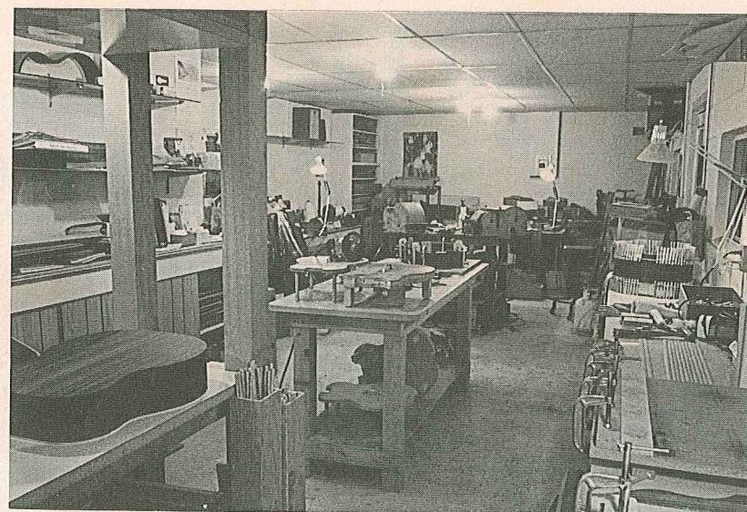
This is the gluing area showing some of the tools and jigs James uses as well as a few guitars in various states of completion.
