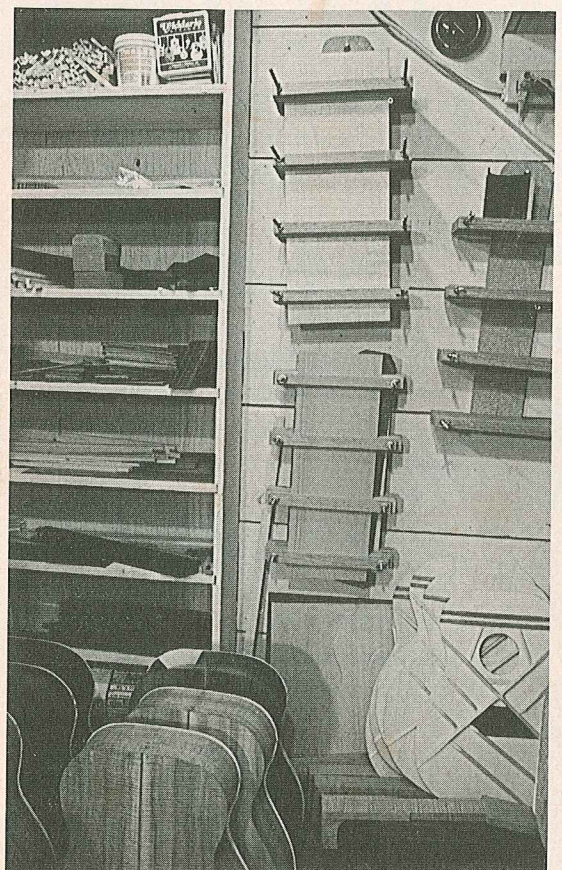
The dehumidifying room. The guitar pieces are kept here before and after gluing. The humidity is a constant 34%.
