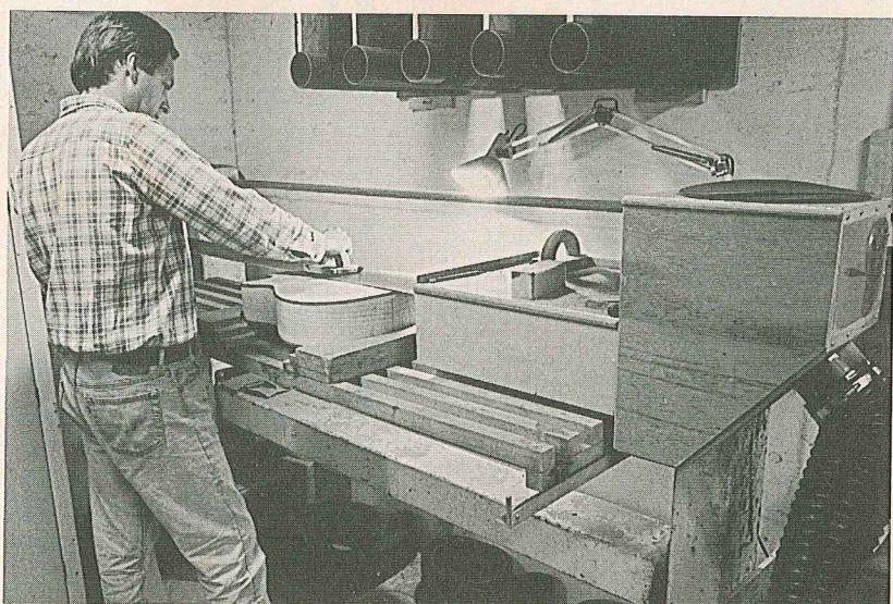
James built this specialized tool for sanding the tops and backs of the guitars. Over the years he has made a number of sanding machines.
